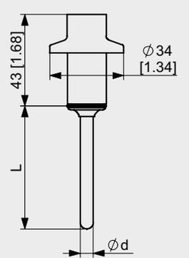
M01 | PHARMadapt ESP G3/8" Überwurfmutter, Ø 3 mm
