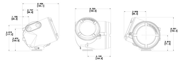
4700 transmitter - aluminum painted housing integral installation
