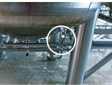
For the feed, ITM-51 is used as a "remote sensor". The measuring point at the pipe lowering ensures optimum product contact. For on-site control with easy access, the measuring unit with display is mounted separately. At the outlet, the compact version of the ITM-51 is a perfect design.
