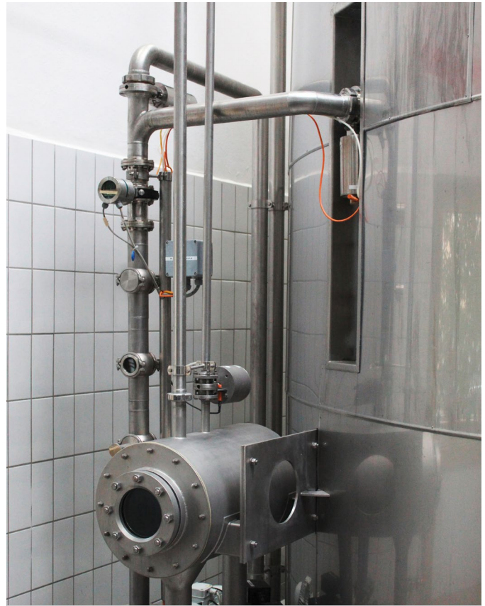
Turbidity measurement and active process control in the lauter tun with ITM-4
